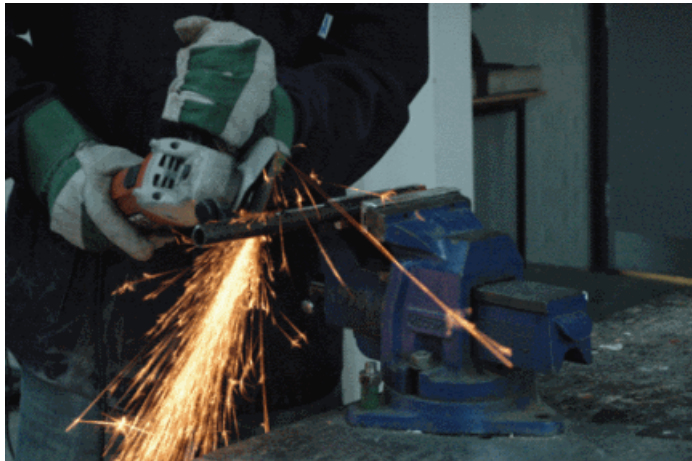
Grinding Hand Held Firearms for Decommissioning, tp Prepare for Transfer to the Foundry
